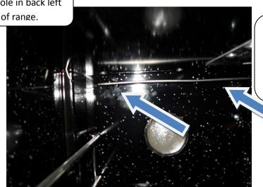
Thermostat probe is secured to back of cavity by 2 clips that can be removed by squeezing
