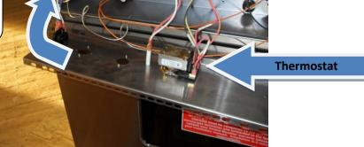
Thermostat enters oven cavity thru hole in back left corner of range.
